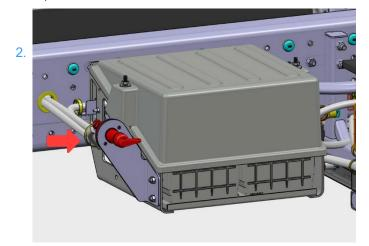
Disconnect the Manual Service Disconnect (MSD) on Battery Management System module (BMS). Shown as position #6 on the **overview picture**.
