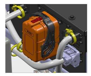
After these two (2) steps are done, there is no 'live' High Voltage circuit remaining in the chassis components. The batteries and cables from the BMS #6 to the Batteries #1 and #2 are still 'live'.
