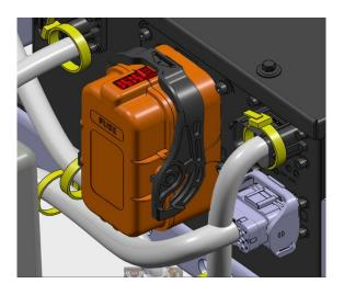
After these two (2) steps are done, there is no 'live' High Voltage circuit remaining in the chassis components. The batteries and cables from the BMS #6 to the Batteries #1 and #2 are still 'live'.
