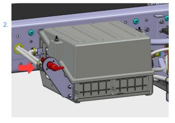
Disconnect the Manual Service Disconnect (MSD) on Battery Management System module (BMS). Shown as position #6 on the overview picture.
